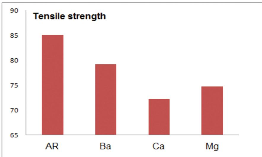
*Fig. 3. Values of tensile strength resulting from tested deacidification treatments*
